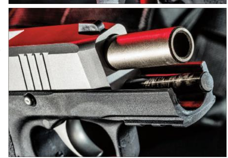
deformation and are therefore more accurate. Their bores also provide a better gas seal for improved velocity. Over the years, I have done extensive testing with both styles on Kahr guns and found that the polygonal barrels are slightly more accurate and the velocities are slightly-and I mean slightly, on the order of 1 percent—faster. The advantages of the polygonal barrel over a conventionally rifled barrel are not something I would pay a premium for. It's a non-issue for me.
